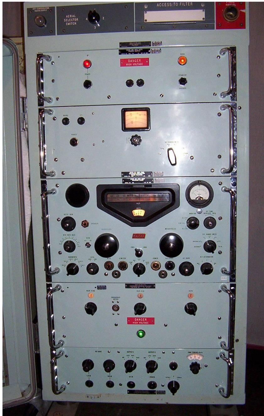
This picture shows all the units powered up. However, as valves are rather hard to get these days, I disconnected the RA117 receiver from all the other units and use it as a free-running set. The bandwidths on this receiver go from 13kHz down to 100hz. The latter being ideal for receiving distant CW signals during a contest pile up. SSB signals can be finely tuned using the BFO. I normally use this set in conjunction with either my Kenwood or Yaesu transceivers.
