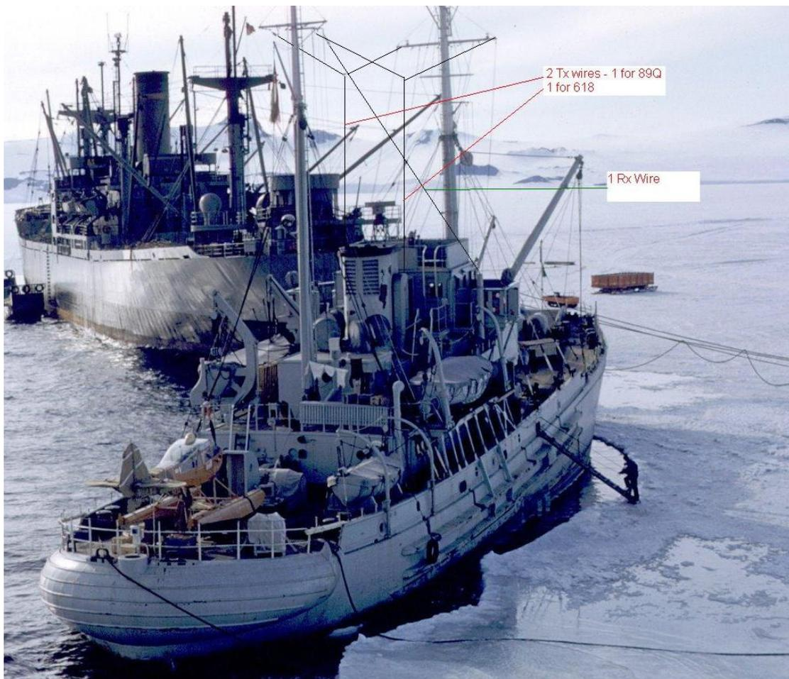
The W/T Office was approximately midships on 1 Deck - the Receive wire can be seen feeding into the Office, starboard side, forrard. The two transmitting wires feeding into the Office, either side of the funnel.
