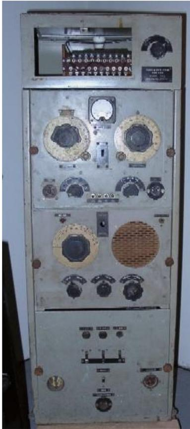
TV5 500-3000 kHz 200 watts (another source states 15w) CW/MCW/AM transmitter/receiver
