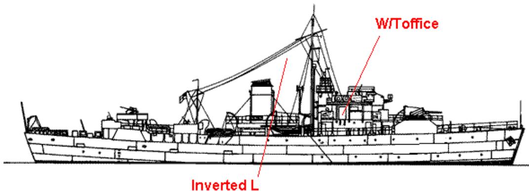
No equipment details for this class of ship, Bird Class (Tui, Moa and Kiwi) or the Isles Class (Inchkeith, Killegray, Sanda and Scarba). However, small ships such as minesweeping trawler corvettes were known to have transmitter/receivers as follows:
