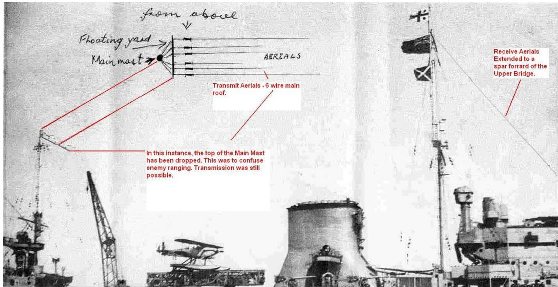
HMNZS Achilles (picture courtesy Ken Shankland, former POREL) showing main roof with the floating yard of the Mainmast dropped. Both masts were the same height which made it easy for enemy gunners to range in on. To help confuse ranging, the mainmast upper yard was able to be dropped slightly and in this position, transmission was still possible. Three receiving aerials went from the Foremast to spars forward of the Bridge and bridge wings.
