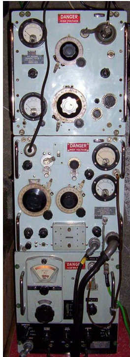
618L on top, 618H in the middle and CAS receiver on the bottom. Power supply normally sat on the deck underneath the bench.
